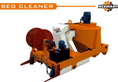
By means of a two lateral scrapers system or brushes, a grinder and a powerful vacuum, it cleans in an efficient and fast way any kind of production bed surface.
